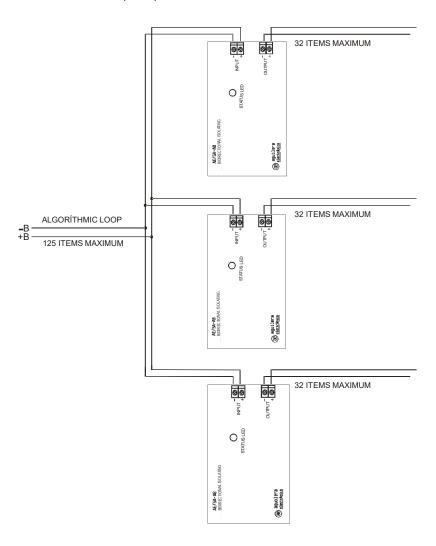
3.- An installation is allowed mixing the above two types of facility, provided the maximum number of items connected after an isolator in open loop or between isolators in closed loop is 32.
